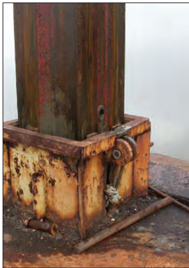
Photos showing spud with securing pin lying alongside (left) and with securing pin inserted (right).
