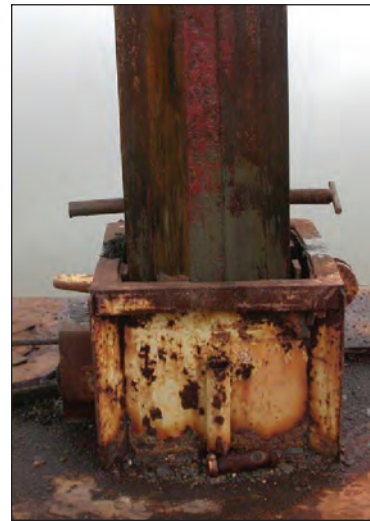
Photos showing spud with securing pin lying alongside (left) and with securing pin inserted (right).
