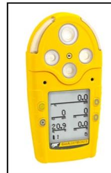
Test for oxygen, combustible gases and hydrogen sulfide prior to opening tank and entering.
